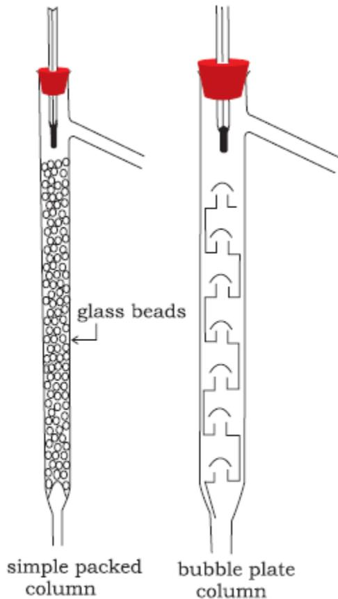
**Fig.12.7** Different types of fractionating columns.
