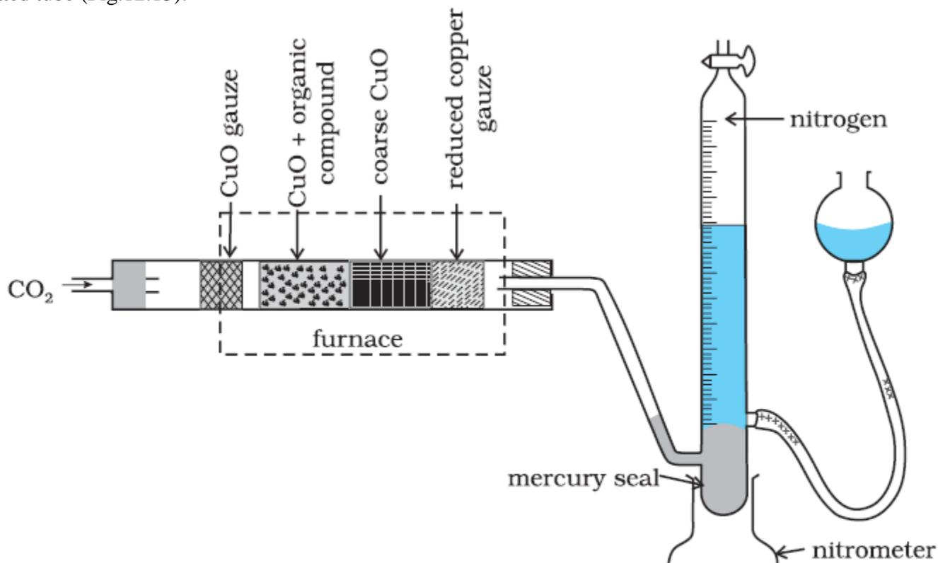
**Fig.12.15** Dumas method. The organic compound yields nitrogen gas on heating it with copper(II) oxide in the presence of CO<sub>2</sub> gas. The mixture of gases is collected over potassium hydroxide solution in which CO<sub>2</sub> is absorbed and volume of nitrogen gas is determined.
