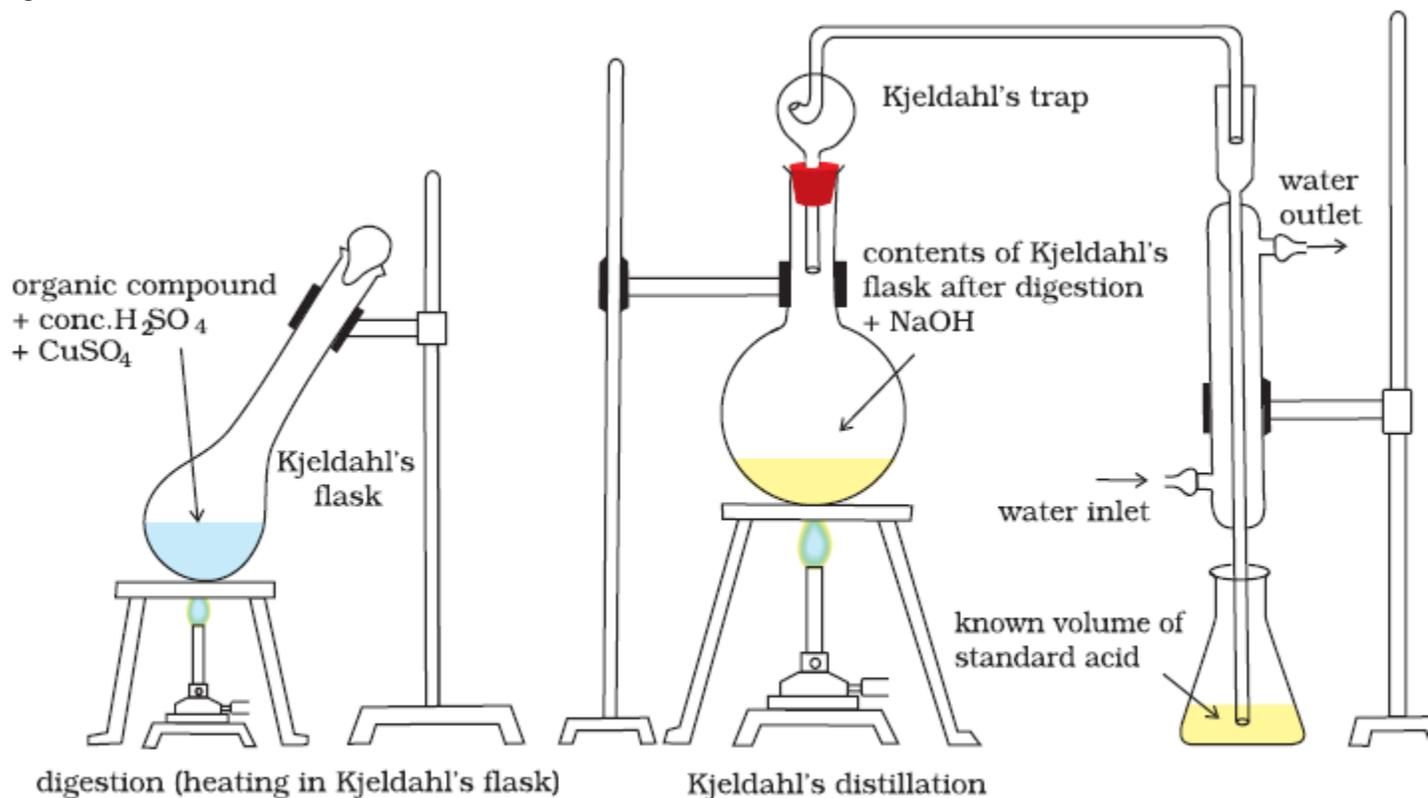
**Fig.12.16** *Kjeldahl method. Nitrogen-containing compound is treated with concentrated  $H_2SO_4$  to ammonium sulphate which liberates ammonia on treating with  $NaOH$ ; ammonia is absorbed in known volume of standard acid.*
