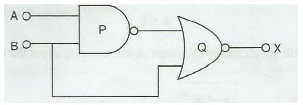
(ii) Write down the output at X for the inputs A=0, B=0 and A=1, B=1.
