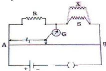
8. In a meter bridge balance point is found at a distance  $l_1$  with resistances R and S as shown in figure. When an unknown resistance X is connected in parallel with resistance S, the balance point shifts to a distance  $l_2$ . Find the expression for X in terms of  $l_1$ ,  $l_2$  and S.
