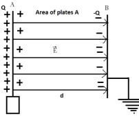
When charge +Q is given to the insulated plate, then a charge –Q is induced on the nearer face of the other plate and +Q is induced on the farther face of the other plate. As this plate is earthed, the charge +Q being free and flows to the earth.
