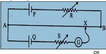
Using a neat connection diagram explain how potentiometer can be used to find the internal resistance of a cell.
