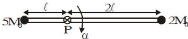
Applying torque equation about point P.
