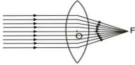
Object at infinity. Image at F on the other side of lens.
