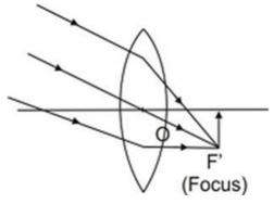
Object at infinity, rays parallel to themselves but not parallel to principal axis. Image is formed at F', the focus on the other side of lens. Object beyond 2F. When the object is beyond 2F, a real, inverted, diminished image is formed between F and 2F.
