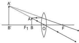
Object between F and C; a virtual, erect, magnified image is formed on the same side.
