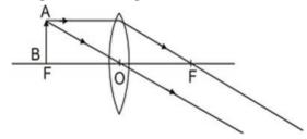
Object at F, a very highly magnified, real, inverted image is formed at infinity.
