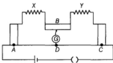
The figure shows experimental set up of a meter bridge. When the two unknown resistances X and Y are inserted, the null point D is obtained 40 cm from the end A. When a resistance of  $10\Omega$  is connected in series with X, the null point shifts by 10cm.
