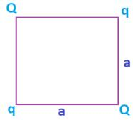
Find the (a) resultant electric force on charge Q and (b) potential energy of this system.
