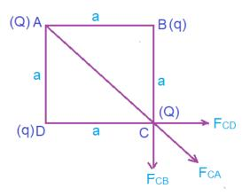
Electric force on charge Q at corner C due charge q at corner B,
