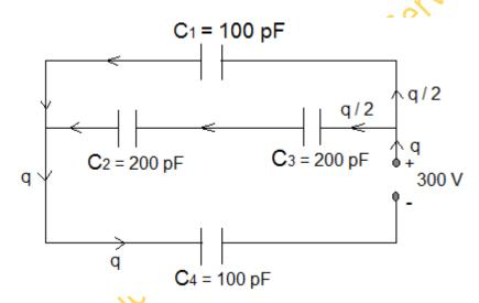
(a) Equivalent capacitance of  $C_2$  and  $C_3$  is
