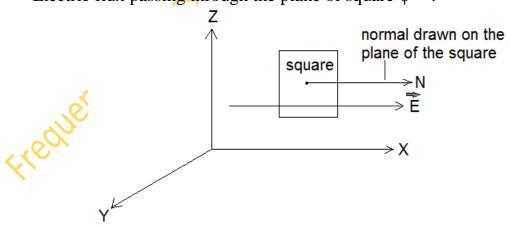
Since, the plane of the square is parallel to the y-z plane and direction of electric field is along X- axis. Therefore, angle between the normal drawn on plane of square and direction of  $\vec{E}$  is  $\theta = 0^{\circ}$ .
