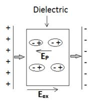
When a dielectric is placed in an external electric field of intensity  $\overrightarrow{E_{ex}}$  then some molecules of dielectric are polarized.
