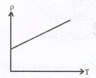
The very weak dependence on temperature of Nichrome, it is used to make standard resistance coil.
