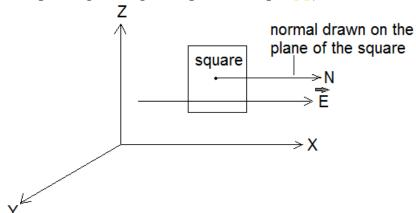
Since, the plane of the square is parallel to the y-z plane and direction of electric field is along X- axis. Therefore, angle between the normal drawn on plane of square and direction of  $\vec{E}$  is  $\theta = 0^0$ .  $\therefore \phi = EA \cos \theta = 3 \times 10^3 \times 10^{-2} \times \cos 0^0 = 30 \text{ Nm}^2\text{C}^{-1}$ .
