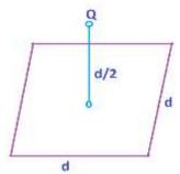
(b) If the point charge is now moved to a distance 'd' from the centre of the square and the side of the square is doubled, explain how the electric flux will be affected.
