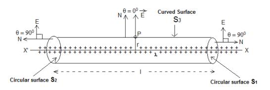
Suppose an infinite long wire is placed in air of linear density of charge  $\lambda$ . We have to calculate electric field intensity at point P at distance r from wire. For this, we imagine a cylindrical closed surface of length *l* and radius r. The point P is situated on this surface as shown in the figure.
