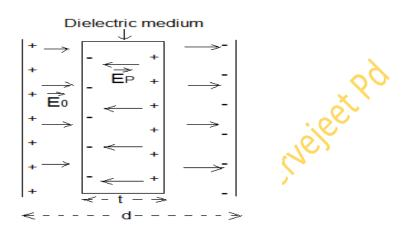
Suppose a dielectric medium of permittivity k and thickness t is placed in between plates of capacitor, where t < d.
