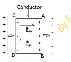
When a conductor ABCD is placed in an external electric field of intensity
