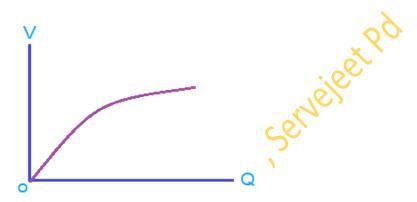
Initially the graph between V and Q is a straight line. But, beyond a certain stage, charge from plate of capacitor starts leakage and V does not increase with increase of Q.
